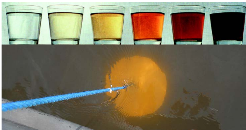
Figure 1. Example of a dilution series of water samples with increasing CDOM content (SLU, Sweden) and a photo of taking a Secchi depth in water with a high CDOM content.
