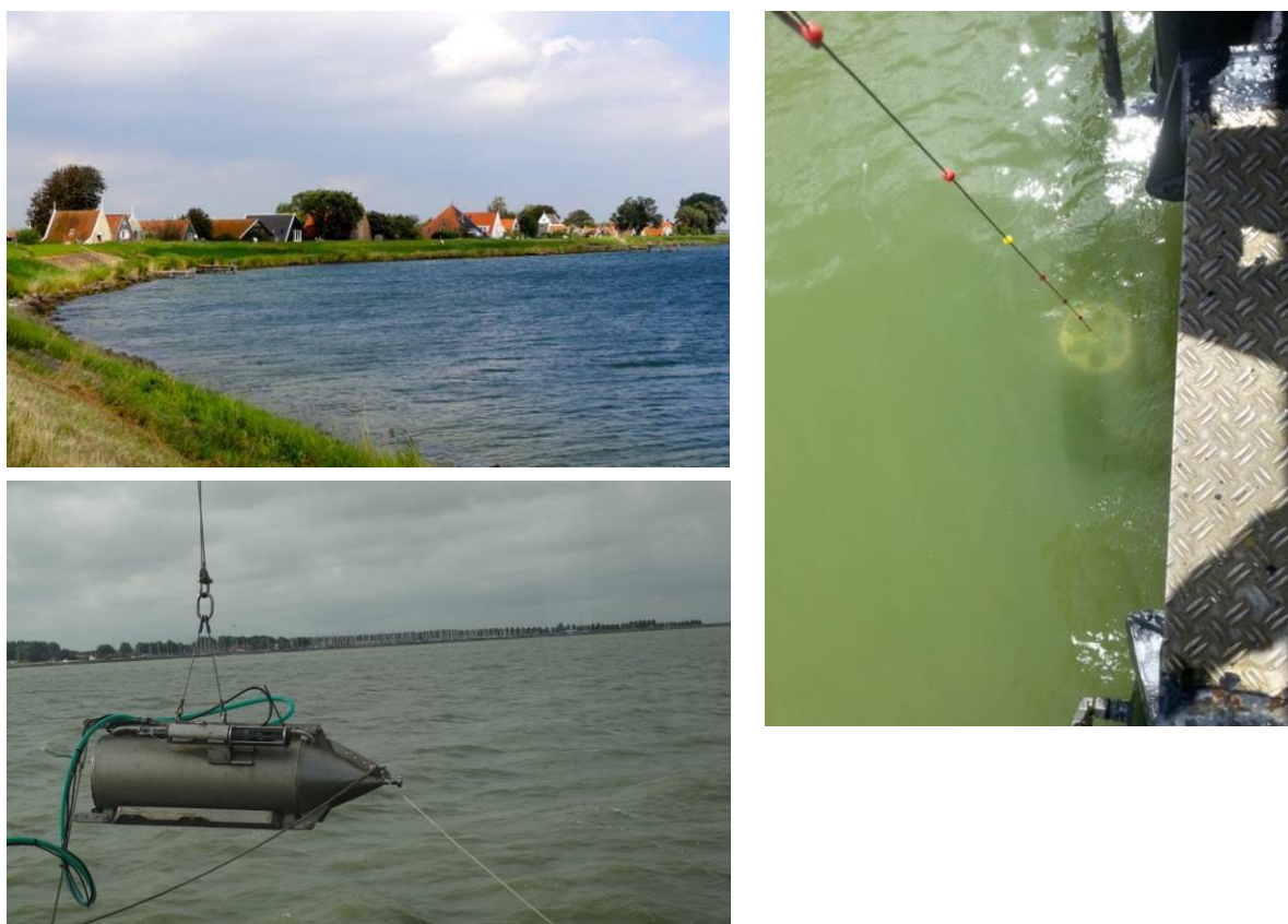
Figure 3. Photos of Lake Markermeer. Top left: dikes surround Lake Markermeer. Right: Secchi disk reading showing the high reflection but low transparency. Bottom left: fieldwork at Markermeer, in the background a harbour full of recreational sailing boats can just be seen.
